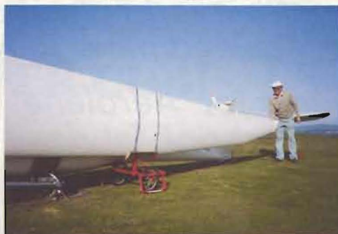
4. The wing is dropped into the holder and strapped in.
