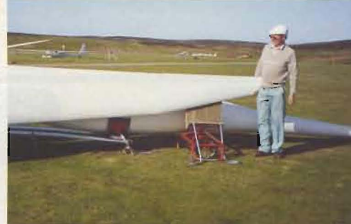
3. The complete unit is placed alongside the fuselage and the wing is pulled out of the trailer.
