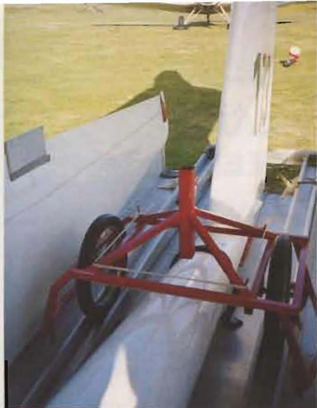
1. The carriage is stowed over the fuselage in the Cobra trailer.
