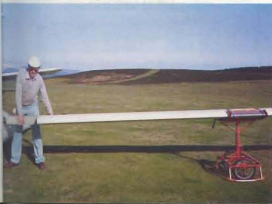
6. The wing is turned flat and the root inserted in the fuselage.
