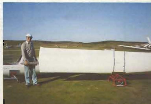
5. The wing balances and can be wheeled around easily – no lifting.
