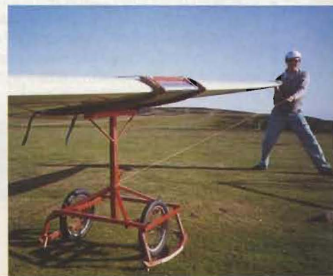
8. Adjusting the height from the tip.
